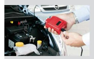
Battery charge state and test functions can be read off easily via the LCD display.
