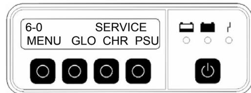
When the "CHR" button is pressed the charger switches to the submenu "Charging function". Here it is possible to define limits for the adjustment ranges for the charging parameters. This makes it possible to allow changes to the charger settings only within extremely close limits to prevent damaging particularly sensitive components in the vehicle with improper settings.
