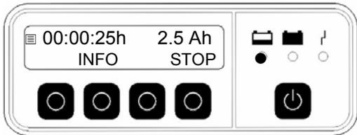
After the battery is completely charged the charger switches over to retention charging.
