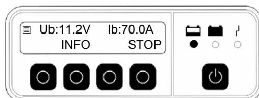
The momentary battery voltage  $U_b$  and charging current  $I_b$  are indicated permanently in the upper line. Pressing the "INFO" button displays the charging time already expired as well as the quantity charged. The display automatically returns to the standard display after 3 s.
