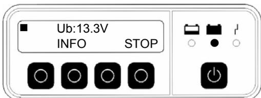
The charging operation can be terminated at any time by pressing the "STOP" button. The charger then returns to the basic menu "Charging".
