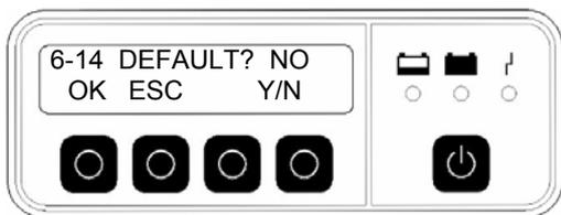
The default answer here is "No", meaning that the charger is not set back to the default settings when the "OK" button is pressed. It is possible to switch to "Yes" with the "Y/N" button.
