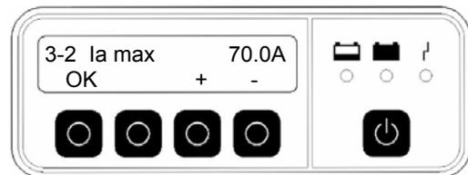
This setting can be saved temporarily in the "TMP" memory. However permanent storage in special programs S1, S2 or S3 is also possible with the "+" and "-" keys.
