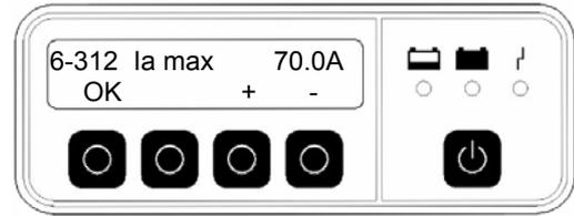
The values are then saved. However this operation can be circumvented by pressing the "ESC" button. The charger returns to the basic menu "SERVICE". From here it is possible to go to the 24V parameter range by pressing the "24V" button.
