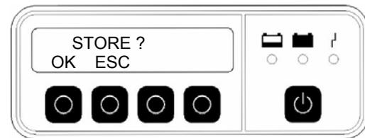
The changes can be saved by pressing the "OK" button again. Press the "ESC" button to delete the changes; the program returns to the basic menu "SERVICE".
