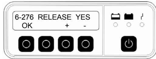
It is possible to switch back and forth between "Yes" and "No" with the "+" and "-" keys. After confirmation with the "OK" button the 24V function is enabled or disabled.
