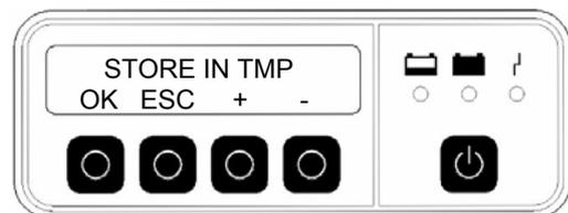
The save operation can be confirmed with the "OK" button or the entire procedure can be aborted with the "ESC" button. Successful storage is confirmed by the display "SAVED". The display then returns to the basic menu "PSU".
