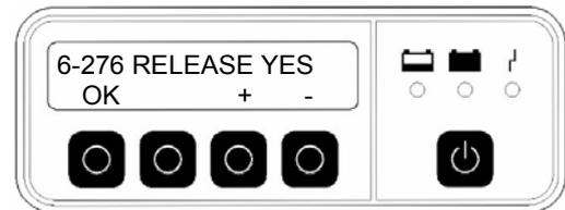
It is possible to switch back and forth between "Yes" and "No" with the "+" and "-" keys. After confirmation with the "OK" button the 24V function is enabled or disabled.
