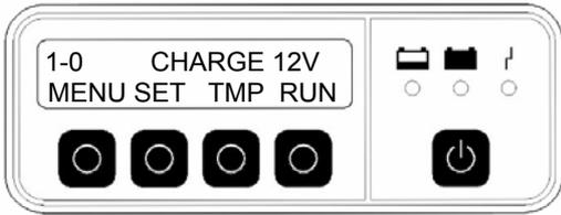
Naturally one of the standard settings ("WET", "AGM", or GEL") can also be selected now; the changes remain stored in "TMP" until the charger is switched off.
