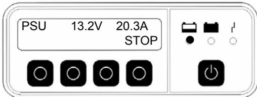
The momentary values for the output voltage and the output current are permanently visible on the display.
