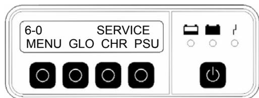
When the "PSU" button is pressed the charger switches to the submenu "PSU function" Here it is possible to define limits for the adjustment ranges for the external power supply parameters. This makes it possible to allow changes to the charger settings only within extremely close limits to prevent damaging particularly sensitive components in the vehicle with improper settings. It is also possible to completely disable the 24V function.
