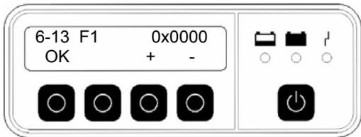
The last ten fault messages F1 through F10 can be viewed by pressing the "+" and "-" keys. They are output in hexadecimal numerical format. The meaning of the most important codes is explained in Chap. 8.
