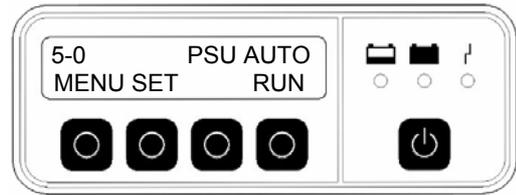
The possibilities for adjustment are limited here to the maximum output current.
