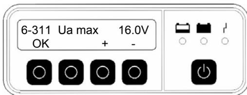
Pressing the "OK" button switches to the next parameter, the maximum value for the output current.
