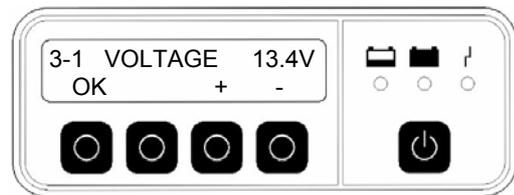
Press the "OK" button to set the maximum output current.
