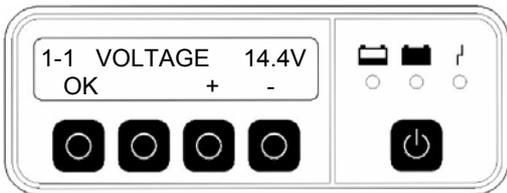
Press the "+" and "-" buttons to change the value in increments of 0.1 V. Press the "OK" button to continue to the next parameter, the value for the charge retention voltage U2:
