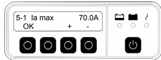
Any change made can be confirmed with the "OK" button and remains permanently stored, i.e. the next time the charger is switched on the value set here is used again.
