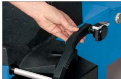
The gauge arm is provided with a patented wheel weight clamp which keeps the wheel weight in the correct position during weight placement.
