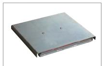
The side-slip tester is designed to measure toe of the vehicle under test immediately. No additional tests are necessary as the testing plate is positioned directly in front of the suspension tester and the vehicle simply rolls over. The data automatically detected supplies a sound diagnostics of toe-in and toe-out. The measured value is read out in 0 +/- 20 mm/m.
