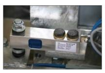
The features to be tested are detected by means of well-proven strain-gauge type load cells. This wear-free measuring system ensures reliable and error-free measurement of the forces produced.
