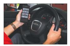
The optional IR remote control unit can be used to control the testing equipment from driver's seat at the entire discretion of the operator, e.g. by starting the brake tester only, or by conducting the tests in the sequence he prefers.
