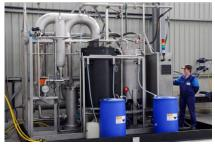
Because of its concern for the environment, CHIMIREC PPM has developed a solution for regenerating cooling fluids and bringing a new life to this waste. After being collected and sorted, the cooling liquids undergo a physical treatment by fine ultrafiltration in order to purify and clarify the used diluted glycol. Cooling liquids are classified as being hazardous industrial waste because they contain ethylene glycol and various additives. They can pollute our environment in the event of a
