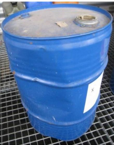
A photograph of a blue metal drum sitting on a metal grate. The drum has a large, shallow, wide dent on its side.                                                              | Großflächige, weiche Delle ohne stärkere Knickbildung, kein Transportverbot.                     |
