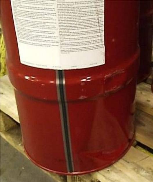
A photograph of a red metal drum with a white label on top. A vertical metal rod is positioned against the side of the drum, creating a soft, shallow dent in the metal surface. | Weiche Delle, seitlich, kein Transportverbot erforderlich, Ware darf weitertransportiert werden. |
