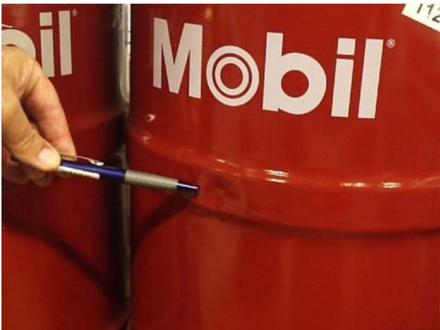
A close-up photograph of a red metal drum with the 'Mobil' logo. A hand is using a blue pen to scratch the surface of the drum.                                                 | Leichte Beschädigung, Fass darf weiter transportiert werden                                      |
